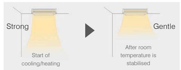
In addition to the conventional 4 fan speed settings, units are now equipped with an Automatic Air-Speed Adjustment Mode. This setting automatically adjusts the air-speed to conditions that match the room environment. At the start of heating/cooling operation, the airflow is set to high-speed to quickly heat/cool the room. When the room temperature reaches the desired setting, the airflow speed is decreased automatically for comfortable heating/cooling operation.
